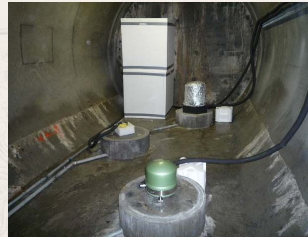
Figure 87: The broadband seismometer at Po Shan Seismograph Station located inside a deep tunnel.
