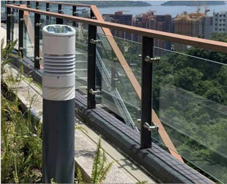
Figure 52: “Bollard type automatic weather station” developed in-house by the Observatory.
