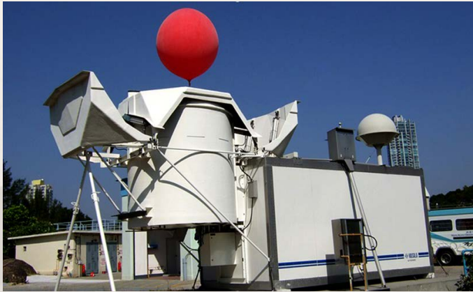
Figure 57: The fully automatic upper-air sounding system was commissioned at King's Park Meteorological Station in 2004, the first of its kind in Southeast Asia at that time.
