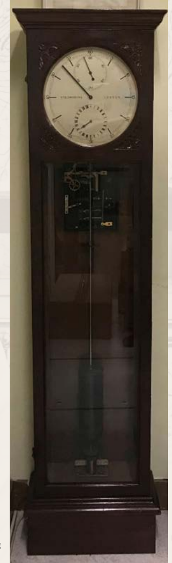
Figure 63: Synchronous standard pendulum clock providing time service in Hong Kong from 1950 to 1966.
