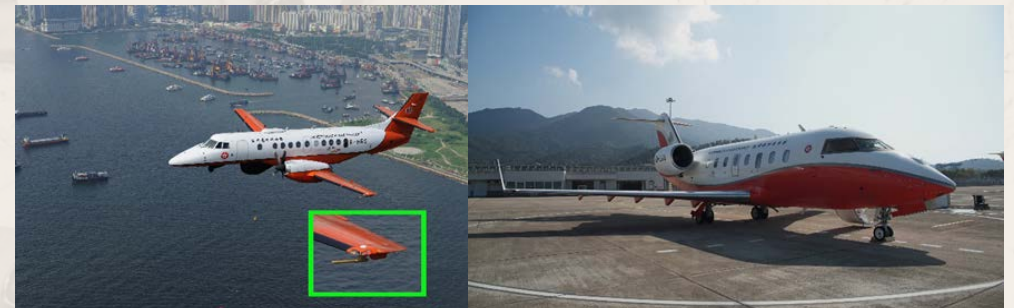
Figure 61: The old and new fixed wing aircraft operated by the Government Flying Service. Since 2011, the Observatory has been making use of them in many occasions to collect meteorological data on tropical cyclones over the South China Sea by flying into the tropical cyclones. A dropsonde launching system was installed on the new fixed wing aircraft for collecting weather data along the vertical direction.
