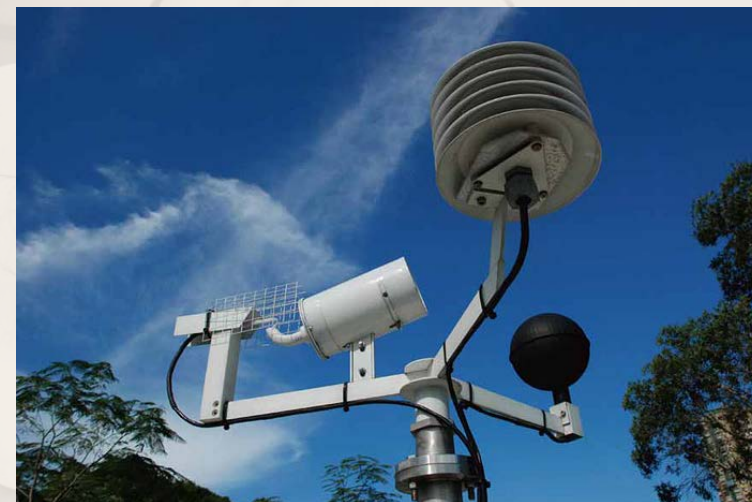
Figure 51: "Heat Stress Monitoring System" developed in-house by the Observatory.
