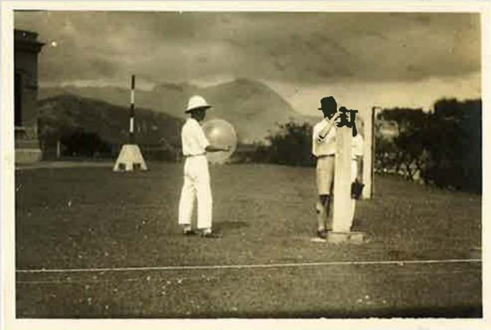
Figure 19: Staff of the Observatory launching a pilot balloon at the Tsimshatsui Headquarters in the 1930s. In the photo, the staff on the left was holding a pilot balloon, while the staff on the right was responsible for operating the theodolite to record the balloon's azimuth and elevation angle, for calculating the upper-air wind speed and wind direction. (Photo courtesy of the family of Mr G S P Heywood, former Director of the Hong Kong Observatory)
